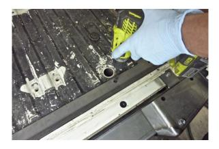
Drill the mounting hole in the vehicle floor using a 7/16" drill bit.
