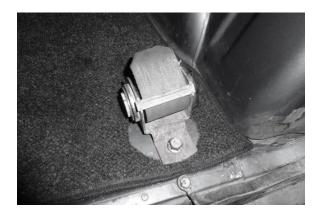
Remove both rear seat belts using a 14 mm socket.
