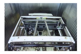
Once you are sure all the pieces are in the correct place, tack weld all the joints not done previously. Be sure to protect all painted body parts, plastic accessories, interior upholstery, etc. from sparks and heat associated with the welding process. A good way to protect vehicle components is using a non-flammable blanket or deflective paper.
