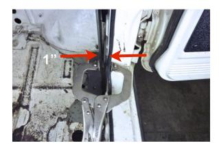
Work with pieces #7 and #8 until they are 3" both sides of center in the front and 6" both sides of center in the rear. Also check to see that piece #6 is parallel (equal distance on both sides) to the windshield assembly. Once you are satisfied that pieces #6, #7 and #8 are positioned properly, tack weld them into place.
