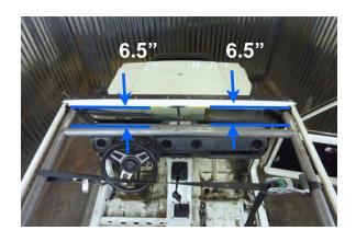
Piece #6 should be equally distanced away from the windshield assembly. We recommend it being about 6.5 inches to begin with. This distance will likely change in the next few steps. But whatever the distance, it should be equal on both sides.
