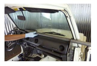
Insert the dash bar (#3) through the side brackets as shown.
