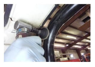
Remove the paint from the existing roll bar using an angle grinder or buffing wheel. This is done to insure a clean weld.
