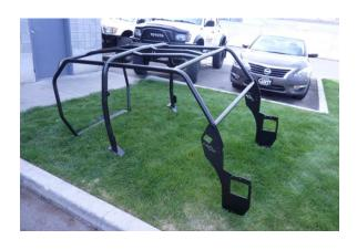
If you painted the sport cage outside the vehicle, wait till the paint dries, reinstall the cage and touch-up any scratches that may have occurred during reinstallation.
