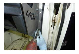
Mark the location of the holes to be drilled with a center punch and hammer.
