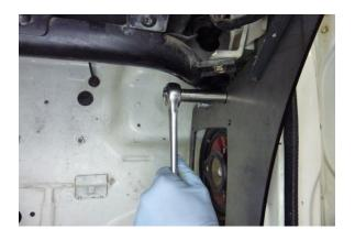
Tighten the (2) bolts 3 or 4 turns ONLY using a 12mm socket. Tighten them just enough to prevent them from coming out. They will be tightened later.
