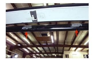
The location of piece #7 and #8 is established by finding the center of the targa bar and measuring out 6" in both directions. Then make marks on the existing roll bar.
