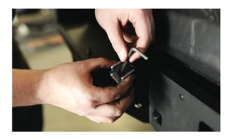
Staring with the hole shown above, use a hex key to install the anchor bracket on the bumper.
