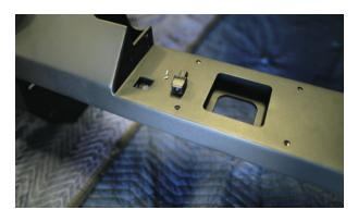
Remove the backup camera from the tailgate and save the 2 small screws that mounted it in place.
