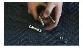
Begin by threading the jam nuts about half way down the threading on the U-bolt.
