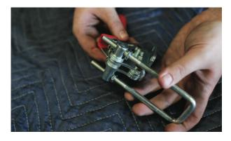
Insert the U-bolt through the rounded end of the swivel bar.
