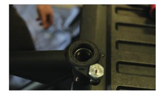
Continue tapping the seal in until it is flush with the housing as shown above. After the seal is installed lightly grease the seal lips.
