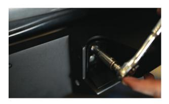
Tighten down both bolts to 12ft-lbs of torque.
