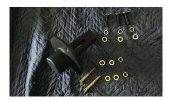
Use the shown hardware to attach the tire mount bracket.
