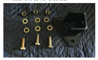
Use the shown hardware to attach the tie carrier base bracket.
