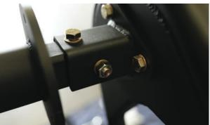
Insert the longer bolt through the side of the base bracket as shown above and secure with washer and nut on opposite side. Torque these bolts to 120ft-lbs.
