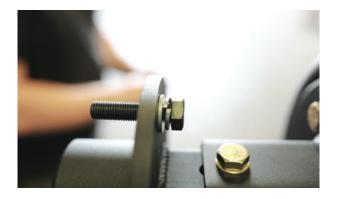
Install the black bolts, lock washers, and flat washers as shown above on all three threaded holes. Torque the bolts to 120ft-lbs.
