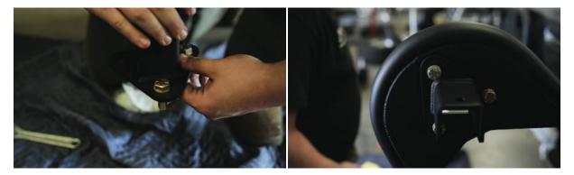
Begin to add the bolts to the bracket and place it on the tire carrier swing arm.
