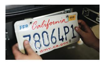
Slide the license plate into the top notch of the bracket, then align the bottom holes with the bolts sticking out of the flip up bracket.
