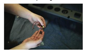
Unscrew the nut from the LED light as shown.
