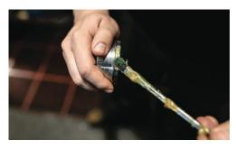
Add a small amount of grease around the lower edge of bearing housing cap for ease of installation and better sealing.
