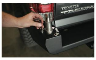
Install the wear plate as shown on the bumper using provided 3/8"-16 button head cap screws.
