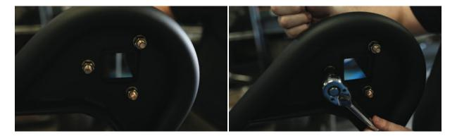
Add the washers and nuts to the back side of the swing arm. Torque the fasteners to 120ft-lbs.
