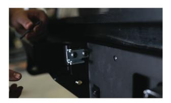
Install the second bolt as shown and tighten both bolts to 18ft-lbs of torque. Repeat on opposite side of bumper.
