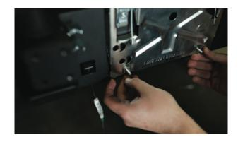
Insert both bolts through the back of the flip up bracket as shown.
