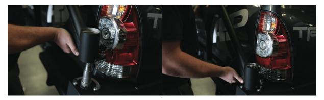
Gently begin to place the swing arm on the spindle. The bearing is seated properly when the arm is able to move down as far as depicted above.
