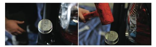
Place grease cap on bearing housing as shown above. Gently tap in grease cap until fully seated on housing.
