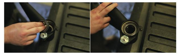
Add a small amount of grease around the lower edge of bearing housing cap for ease of installation and better sealing.
