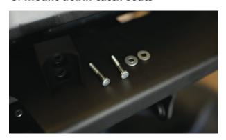
Using the shown hardware to install the delrin catch seat
