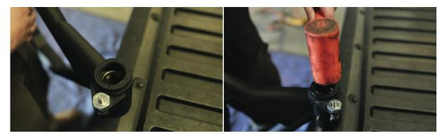
Place the grease seal as shown on the bearing housing and begin to tap it in with a hammer.
