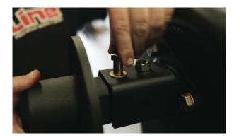
Using the shorter bolt, insert through the top of the base bracket and through the tire mount bracket. Secure with washer and nut.
