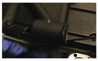
Install the provided Zerk grease fitting on bearing housing as shown. Torque to 15ft-lbs.
