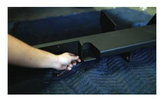
Feed the wires through the shown hole.
