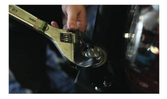
When tightening be sure to align one set of slots in the castle nut with the pin hole on the spindle.
