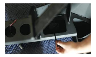
Feed the wire through the large rectangular hole on bumper.
