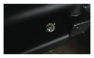
Be sure to put the lock washer between the bolt and the flat washer.
