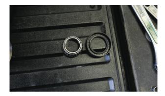
To install the tire carrier arm, begin with the larger tapered roller bearing and the rubberized grease seal.
