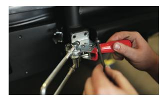
Hold the assembled latch up to the swing arm and begin to add the bolts as shown. Once properly aligned, torque all four bolts to 18ft-lbs.
