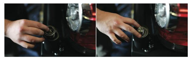
Grease the smaller taper roller bearing, gently insert it into the housing. You may have to lift the swing arm in order to seat the bearing fully.
