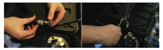
Insert pull pin assembly to flange as shown and use provided nut to secure in place. You may use Loctite here if desired.
