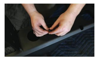
Feed the wire through the nut and proceed to tighten the nut down on the LED light.
