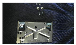
Install the license plate flip up bracket with the hardware shown.
