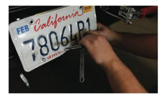
Using another ¼" flat washer and provided ¼-20 top lock nut, tighten the bolts that hold the license plate.
