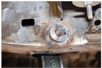
**STEP 24** Weld the shackle mount to the bottom of the frame.
