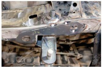
**STEP 28** Finish welding the bottom support plate.
