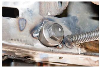
**STEP 21** Weld the support plate to the frame.
