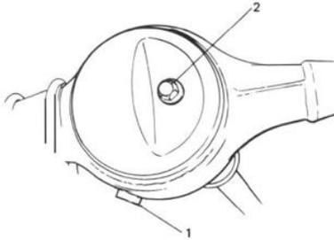
Fig. 16-33 ① Drain plug
