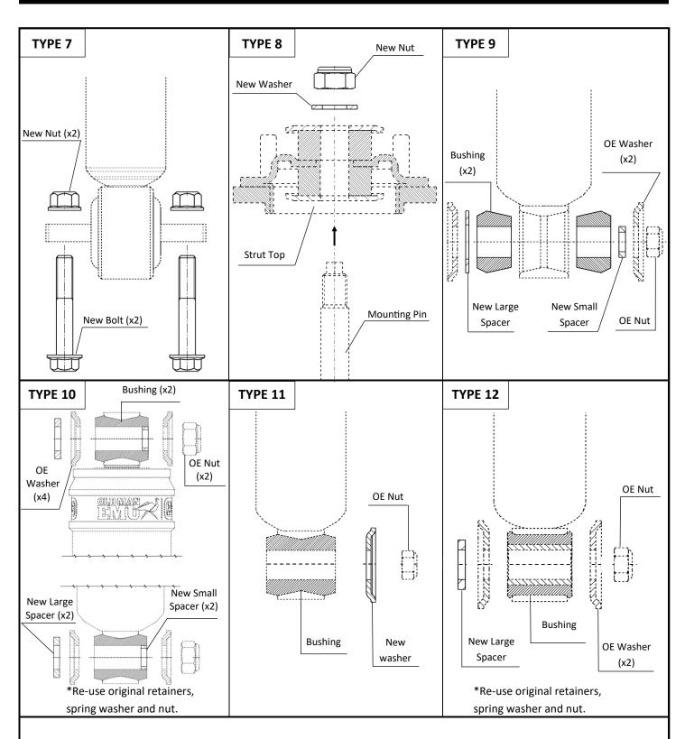
To ensure correct fitment of small mounting parts reference type number on SMP bag to above chart
