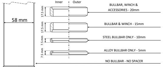
Note internal profile to determine height offset
