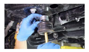
Place one of the supplied differential drop spacers between the bracket and the cross member and install the bolt up through the bracket, the spacer and the cross member.
