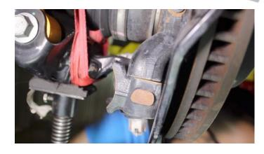
Continue tightening the ratchet strap and raising the under hoist jack stand simultaneously until the ball joint bracket and the steering knuckle come together.
