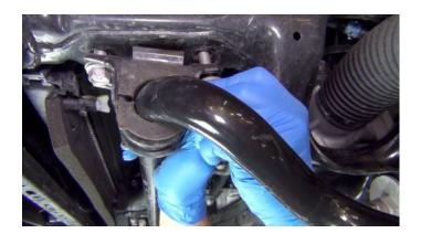
Start the driver side rear sway bar bracket bolt. Leave it loose for now.
