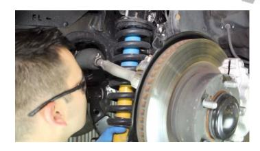
While supporting the shock absorber assembly with one hand, remove the 4th nut.
