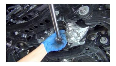
Tighten the driver side differential mount bolt to 89 ft. lbs.
