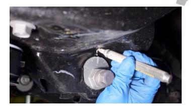
Mark all 4 alignment cams (See Figure 4) so they can be returned to their initial alignment settings. Although these settings will not end up being exactly the same after the alignment, it will help the alignment technician to know where the original settings were.
