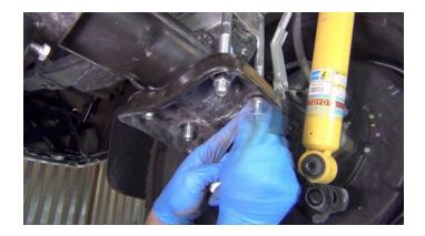
Step 120 Now install the other three washers and flange nuts on the remaining U-Bolt ends.
