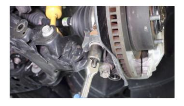
Remove the front lower ball joint bracket bolt using a 22mm socket.
