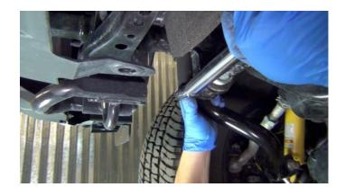
Tighten the (2) passenger side sway bar bracket bolts to 51 ft. lbs.
