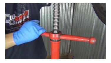
With the supplied spacer block "F" oriented forward and down, place the block on top the spring perch insuring that the locating dowel fits properly, all the way down in the hole. There should be no gap between the spacer block and the spring perch.
