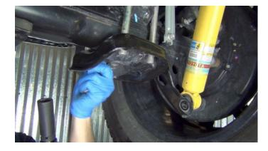
Remove the (4) U-Bolt nuts and washers using a 19mm socket.
