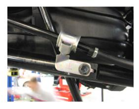
Correct positioning of the park brake cable.
