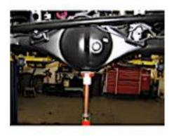
Support the center of the rear axle assembly with a floor jack (or an underhoist safety stand) and raise the rear axle assembly slightly.
