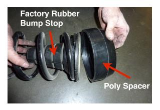
Install the supplied poly spacers on the top of the factory rubber bump stops with the tapered side up.
