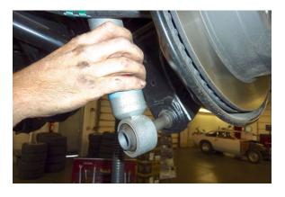
Using the floor jack (or under-hoist Jack stand), lift the rear axle assembly. Then reconnect both rear shock absorbers to the axle. Torque the bolts to 72 Ft. Lbs.
