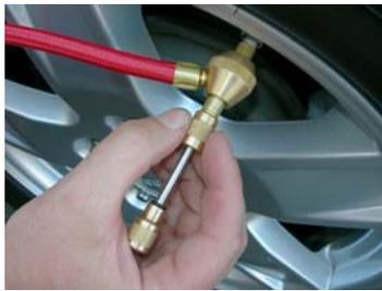
1. With the slide valve pushed forward, thread the valve stem adaptor onto the valve stem in a clockwise direction.
