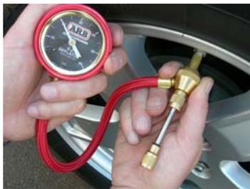
4. Pull out on the slide valve to release air. Push in on the slide valve to stop air and check the pressure. Note, gauge will not show correct pressure whilst deflating.
