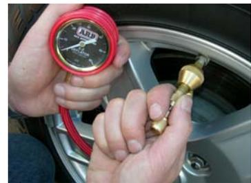
6. Remove the unit by turning the valve stem adaptor in an anti-clockwise direction. Ensure a valve cap is placed on the valve stem to prevent ingress of debris.
