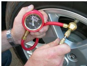
5. When the desired pressure is reached, push the valve core remover in and turn clockwise until the valve seats firmly. Note: Do not over tighten the valve core.
