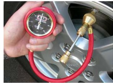
3. When the valve core is removed it will push the core remover out and the gauge will read the tyre pressure.
