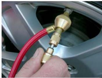
2. Push the valve core remover forward until it engages the valve and turn anti-clockwise to remove valve.
