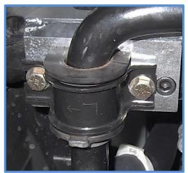
10. Install the sway bar to the threaded holes in the reservoir bracket using the 3/8 x 3/4" bolts and washers provided in the kit. The factory sway bar brackets are side specific and stamped "L" and "R" with an arrow that points toward the front of the vehicle. After the sway bar is mounted to the frame you can reconnect the sway bar links to the steering knuckle.
