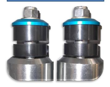
3. For the lower mount place one spacer on the mounting stud (A), then install the rod end followed by the other spacer. Make sure that the spacer is not sitting past the mounting stud (B). Use the factory bolt and tighten to factory specs (C). See photos on next page for proper shock orientation, position shocks accordingly and tighten the nut on the upper mount.
