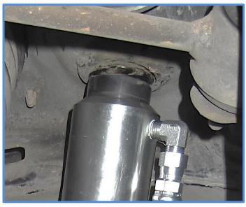
Make sure that the short bushing is toward the cylinder and the taller bushing is on the other side of the upper mount with the anodized washer, flat washer and lock nut.
