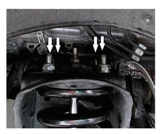
Figure 2: Top mount fastening to frame
