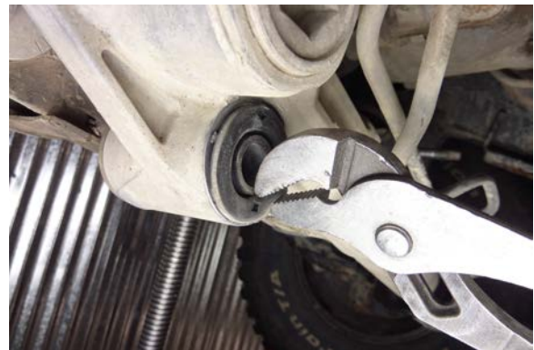
Step 27 Begin removing bushing B by tearing the back side of the bushing away with pliers or cutting it away with a knife.
