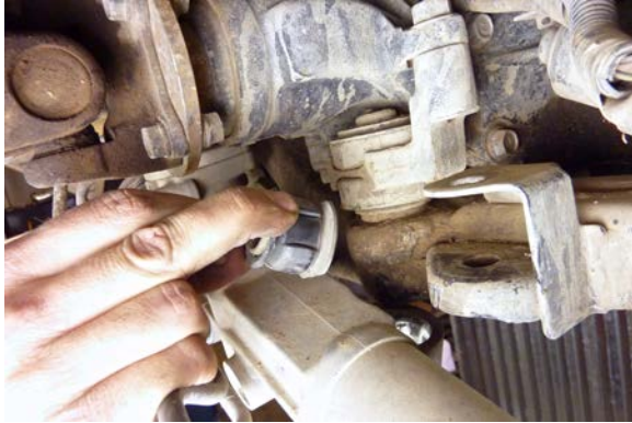
Step 35 Bushings A removed.
