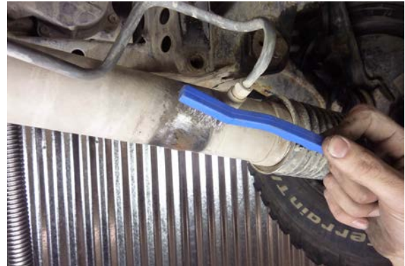
Step 25 Clean any dirt or rust from the bushing C area of the rack with a wire brush.
