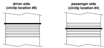
On **4Runner 4x4 KDSS** models, it is recommended that the **driver and passenger side circlips are installed in the same position**. For example, to achieve the highest lift setting of 3.2", the circlips should be installed as follows:
