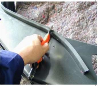
35. Using a sharp knife cut the excess rubber in line with the inside end of the wing. Only cut the inside excess, the other end will be cut when the winch bumper is fitted.
