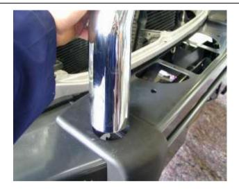
16. Push the top Sahara tube through the hole in the buffer and fasten using the M12 x 40mm bolts, washers and spring washers.
