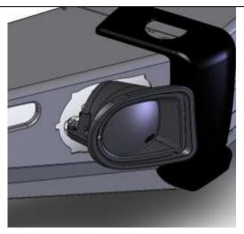
11. Fit fog lamp housings (3163082) into the bull-bar fog lamp cutouts as shown. (RH Shown).
