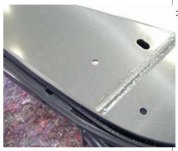
33. Insert the mount strips inside the channel section of the rubber extrusion. Make sure the flap section is on the outer side. Allow generous even amounts of excess at either end of the strip so that it can be trimmed later.
