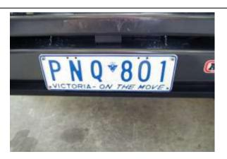
20. Bolt the number plate through the top holes using M6 X 16mm bolts and M6 flange nuts. If desired double sided tape can be used down the sides of the number plate.
