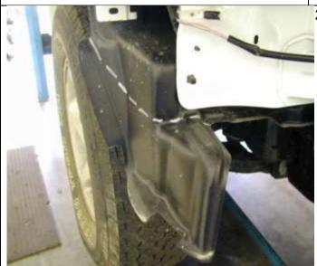
Using sharp scissors or a cutting blade, cut the plastic inner guard as per line shown in the photo. (RH shown).
