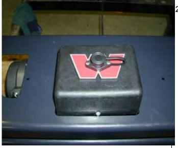
25. Fasten control box assembly to the bar using the M6 x 16mm bolts and flange nuts.
