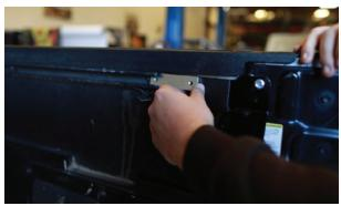
**3.** Using bolts with lock and flat washers, and the help of a friend; position the bed rack and begin to install the bolts. Leave the bolts loos for now.
