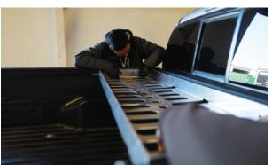
**4.** If the rack is narrower than the bed, drop in the provided spacers until the extra space is filled. Once the spacers are dropped in tighten all the bolts.
