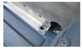
If installing the compressor box on the passenger side, make sure the power connector for the outlet plug is inside the compressor box before tightening lock nuts.
