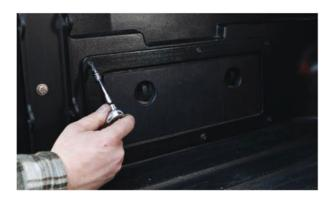
**2.** If you are installing the passenger side AP steel door, remove the (4) screws holding the factory outlet plug to the factory bed storage box.
