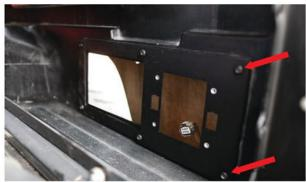
Install longer bolts in these locations for both original bezel and AP bezel.
