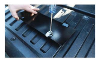
**4.** If you are retaining your original bed box bezel and door, measure 1/2" from the base of the factory box as shown. Extend a line between the measured points around the box. Using a cutoff wheel trim the box along the line. Cut off the (2) plastic alignment tabs on the back side of the bezel as shown in the picture.
