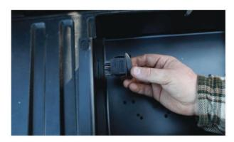
8. If applicable, install the ARB compressor into the box using the existing mounting holes.
