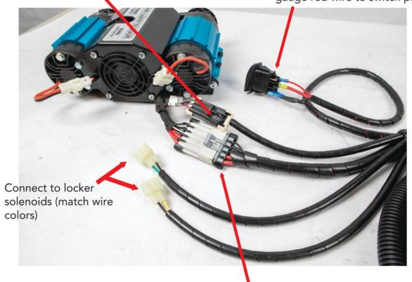
Connect to compressor power connector on compressor
