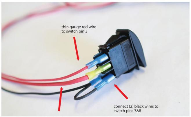
thick gauge red wire to switch pin 2
