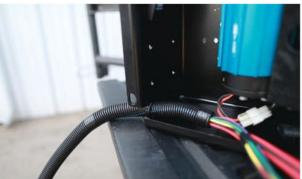
**10.** Connect the necessary connectors of the wiring harness to the connectors on the compressor or locker solenoids. Route the wires for the rocker switch back out of the box through the installed grommet and connect the wires to the appropriate terminals of the rocker switch.
