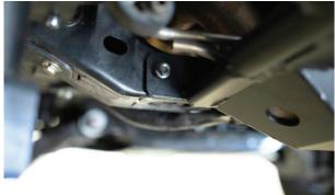
**14.** Reinstall bolt through the skid plate and brake line bracket.
