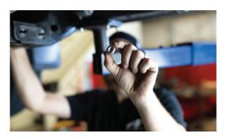
**8.** Put the  $\frac{1}{2}$ " bolts with washer through the center holes of the cross member.
