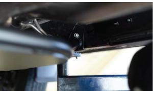
13. Install lock washers on all 4 cross member bolts and secure with nuts.
