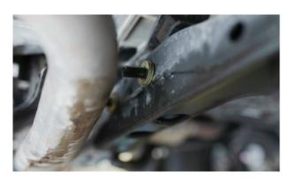
**10.** With the help of a friend or a jack slide the skid plate over the bolts, you may use one of the factory nuts on the cross member bolt to secure it. Eventually the cross member bolts will all get lock washers. It is recommended to proceed through step 14 before fully tightening any bolts.
