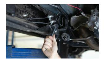
**2.** Straighten the hook at the bottom of the brake line bracket.
