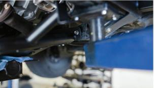
11. Reinstall bolt through the skid plate and brake line bracket.
