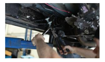
**3.** Remove the bolts holding the small skid plate on the bottom of the transfer case and remove the skid plate.
