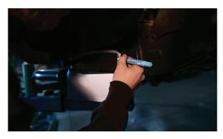
7. Inner fender liner will be marked and cut as shown. A utility knife work best.
