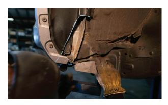
**13.** Once a good fit is achieved it may still be necessary to shape the plate and/or body mount using a hammer after tacking mount in place.
