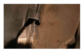
**19.** After cleaning use undercoating to cover the portion of the pinch weld that has been hammered over in order to endure the pinch weld is still sealed.
