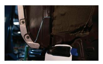
**8.** Mark and cut fender as shown. Cut off wheel on a grinder works well for this. Not all applications will look exactly the same as this picture. Different models may require slightly different fender trimming, but we recommend trying to trim the fender on the same plane that the body mount will be cut. This cut may also need to be adjusted for larger tires. (Vehicle used in instructions is 2017 Tacoma.)
