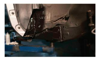
**17.** Cut pinch weld in body as shown. Be careful to not cut all the way through as you will open a hole into the cab.
