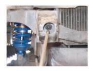
6. Remove factory skid plate from truck using 10mm - 14mm sockets. There are a total of 7 fasteners.
