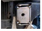
19. Finish welding the brackets into place along the vertical joints only. Weld a little at a time and let cool so as not to over heat the frame rail or catch anything on fire - "follow good welding practices and safety." If you are unsure of your welding skills, have a certified welder make these welds for you.
