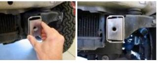
17. If necessary, gently tap the brackets into the frame rails until they are flush with the ends of the frame rails and the surface of the brackets are square to the sides, top, and bottom of the frame rails.
