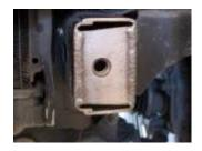
20. Grind the welds smooth and flush to the face of each bracket being careful not to overgrind them weakening the joint or bracket. Grind the ends of the side bumper mounts if you ground off the "errory ting"
