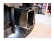
16. Insert the frame end caps with the treaded inserts as shown. the frame end caps are identical and will not fit both the driver and passenger side frame rails. In order for them to fit correctly, position the longer bent side towards the outside of the rails and the shorter bent side towards the inside of the rails. The brackets are designed to fit the irregular shape of the frame rails.
