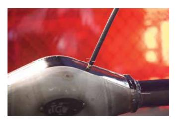
NOTE: If the grommet hole on top is going to interfere with suspension mounting points a one inch diameter hole can be drilled elsewhere in the truss in order to pass the extension hose.
