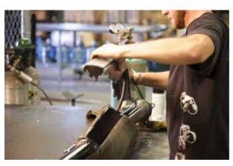
**STEP 8**Install extension hose and clamp onto the barb fitting.
