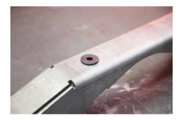
**STEP 10**Place truss onto the housing and run extension hose through the breather hole and grommet.
