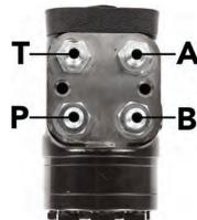
T = Tank A = Left P = Pump B = Right
