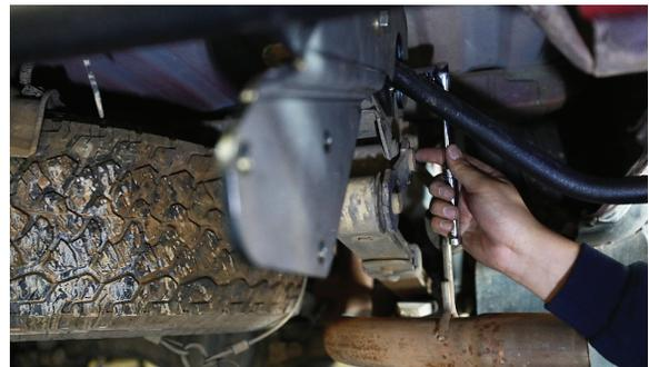
**9.** Tighten the bolts to the hitch
